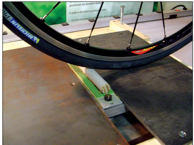
Figure 11. Front wheel about to impact wooden stud mounted on instrumented bump.
