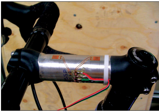
Figure 16. Instrumented stem to measure vertical force on handlebar.
