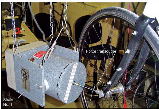
Figure 3. Shaker 1 imposing horizontal force at 30° off bike plane.
