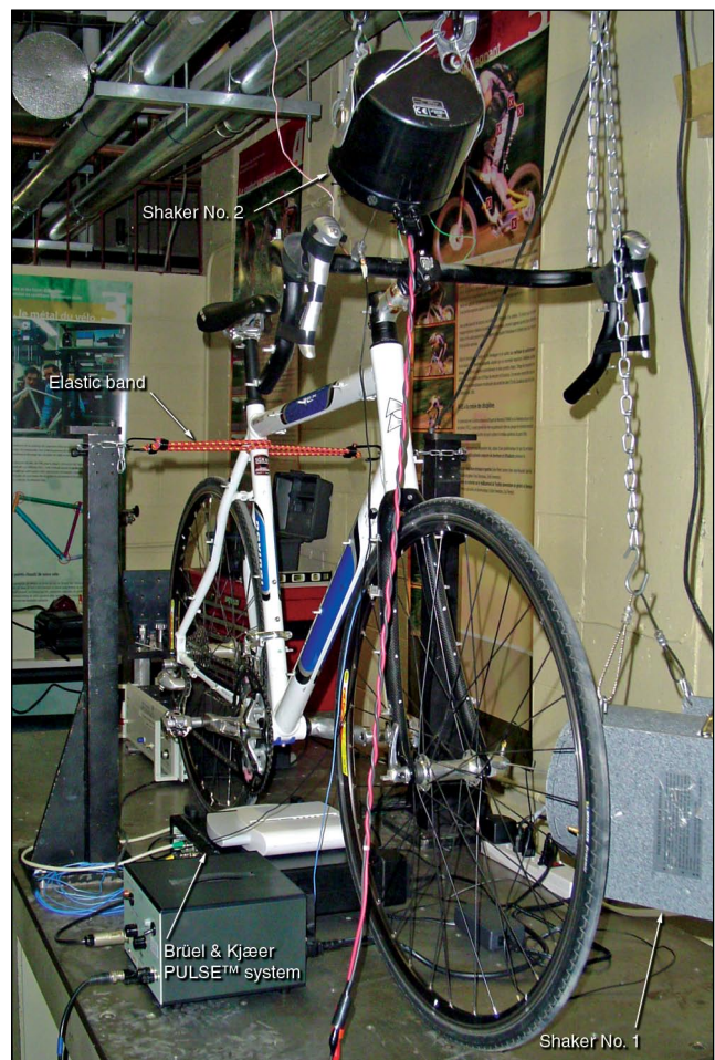
Figure 2. Setup for SIMO and MIMO analyses.
